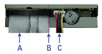
Figure 4 - 31: Cabling a Floppy Disk Drive
